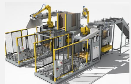
**16 SKID-BASED BOX BOT SERIES PALLETIZERS WITH 6-AXIS ROBOTS ALLOW FOR ROBOTIC PLACEMENT OF PALLETS AND SLIP-SHEETS WITHOUT THE NEED FOR ADDITIONAL FUNCTIONALITY ON THE ROBOT'S EOAT.**
