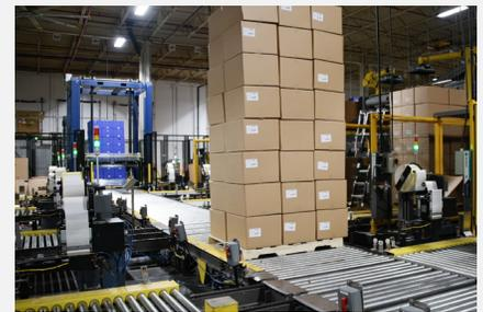
STACKED PALLETS DISCHARGE FROM EACH BOX BOT CELL BUILD STATION ONTO A CENTRALIZED TRUNK LINE THAT CONVEYS TO AN AUTOMATIC STRETCH WRAPPER.
